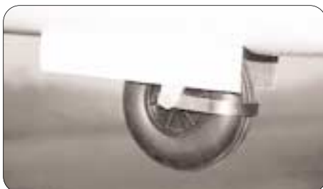
The main wheel doors were reinforced with an overall layer of carbon fibre cloth (left) to produce superbly rigid panels.
