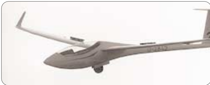
The first landing with main wheel extended and airbrakes fully deployed was straightforward, with no nasty surprises (above).
