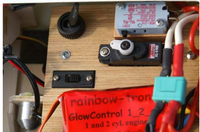
The figure shows the IC servo and the micro switch which is used to start and stop the starter engine.
